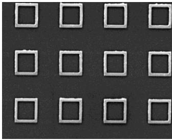
Square lattice ( $4.1 \times 4.1 \mu\text{m}^2$ ) of Permalloy square rings ( $2.1 \mu\text{m}$  side). Nominal width 250 nm. Thickness 30 nm.
