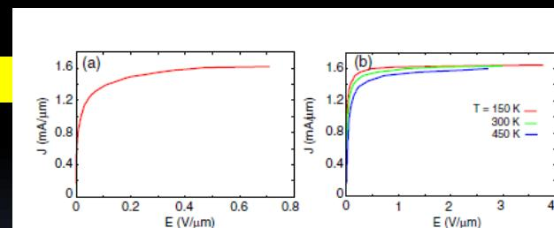
FIG. 2 (color online). The role of the interaction between phonon polaritons in  $\text{SiO}_2$  and free carriers in graphene for graphene field-effect transistor transport. The separation between graphene and  $\text{SiO}_2$  is  $d = 3.5 \text{ \AA}$ . (a) Current density-electric field dependence at  $T = 0 \text{ K}$ ,  $n = 10^{12} \text{ cm}^{-12}$ . (b) The same as in (a) but for different temperatures.
