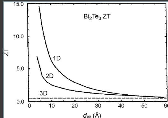
Dependence of  $Z_{2D}T$  and  $Z_{1D}T$  on quantum-well and quantum-wire widths  $d_w$  for  $\text{Bi}_2\text{Te}_3$
