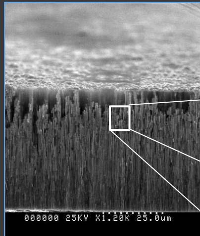
Alumina matrix completely filled. Almost no overgrowth.
