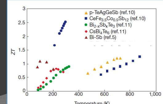
Figure 3 Temperature dependence of  $ZT$  of  $10\text{\AA}/50\text{\AA}$  p-type  $\text{Bi}_2\text{Te}_3/\text{Sb}_2\text{Te}_3$  superlattice compared to those of several recently reported materials.
